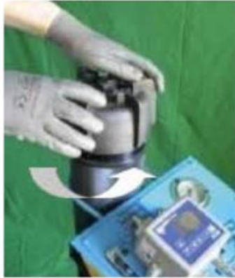
Figure 3 – Unscrew the cover
