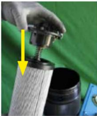
Figure 5 / 6 - Insert the endcap with bypass (Fig. 5) or the possibly selected blind endcap (Fig. 6) in the filter element
