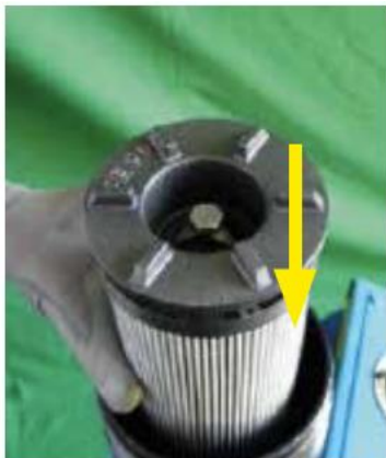
Figure 7 - Insert the filter element into the filter body
